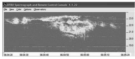
Figure 6 — Radio spectrogram of Jupiter radio noise storm activity. Horizontal lines are weak stations while Jovian signals are seen as the enhanced region between 20.2 and 23.5 MHz. Any resemblance between this emission region and the shape of the starship *Enterprise* is purely coincidental.
