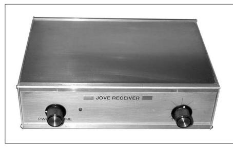
Figure 2 — The Jove RJ1.1 direct conversion receiver is simplicity itself with only two controls – a POWER SWITCH/VOLUME CONTROL and a TUNING knob. Low level audio from the receiver is sent to a computer sound card and also may drive an amplified speaker. The receiver uses a J310 grounded gate RF amplifier followed by the traditional NE602 mixer/ oscillator and high gain audio amplifiers. A varicap tunes the receiver over a 400 kHz range centered on 20.1 MHz.
