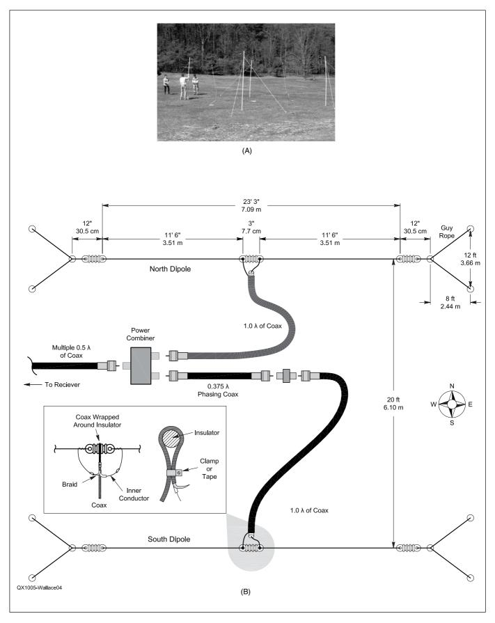
Figure 4 — The Jove dual dipole array. Dipoles are suspended between PVC masts. Signals from the dipoles go to a power combiner and then to the receiver.
